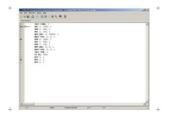
INFO TMCL-PC is a PC based version of the simple-to-use TMCL software. It allows the control of multiple modules via one PC, so that any kind of interaction between the motors and I/Os available on the different modules can be realized. This for example allows the BLDC motor modules to be inter-operated with stepper motor modules.
