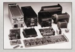
Various low-cost 'open board' units to complete units with built-in power supply module, with KEMA CE/EMC quality mark (KEMA = Testing, Research and Engineering Consultants to the Electric Power Industry). Options available include: encoder interface, analogue input, oscillator, connection network of several units and tracking systems.
