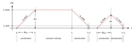
Driving a stepper motor at velocities higher than its physical start stop frequency requires a defined acceleration. For the great majority of positioning applications linear ramping profiles are sufficient.
