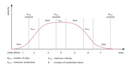
For high speed positioning as well as for handling of jerk sensitive goods or objects with extensive inertia sinusoidal (S-shaped) ramping profiles might be necessary.
