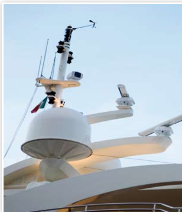
A highly reliable brushless DC motor keeps this satellite antenna on track in a harsh and demanding marine environment.
